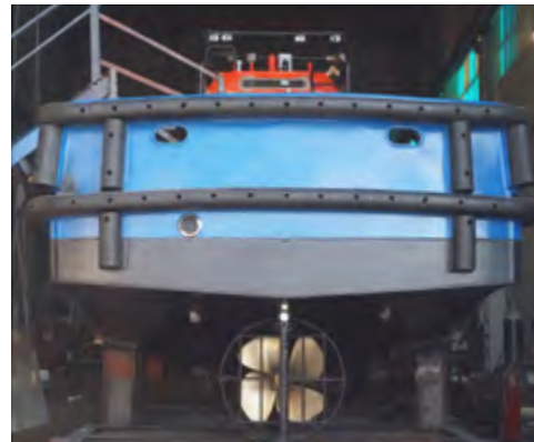
PROPULSION AND CONTROL. 850 mm propeller in nozzle and rudder with high-performance flaps.
