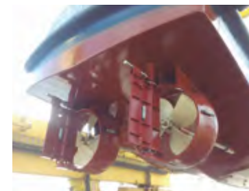
PROPULSION AND CONTROL. 1,050 mm propellers in nozzle. High-performance flap rudder.
