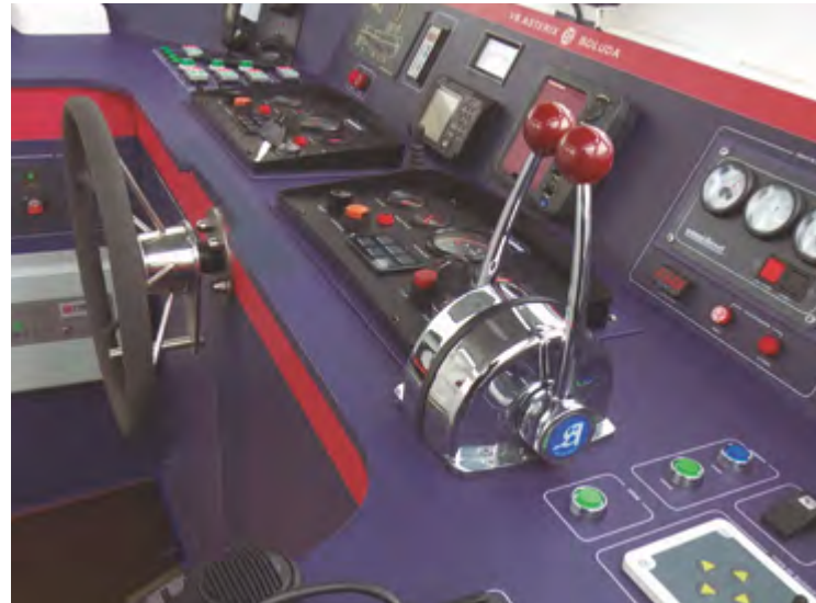
CABIN. Control desk adapted to the operational needs of the ship's crew.
